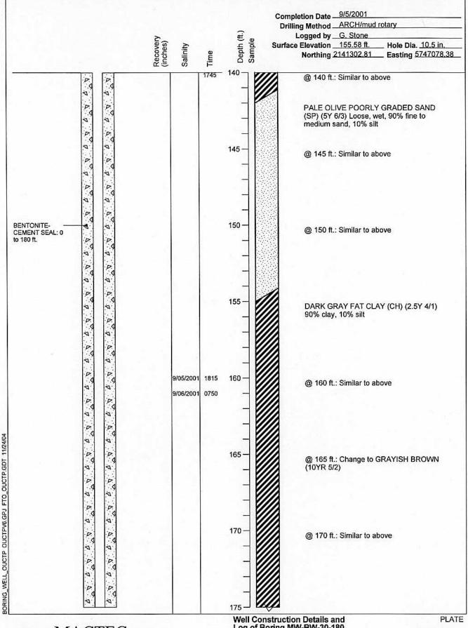
Well Construction Details and Log of Boring MW-BW-30-180
