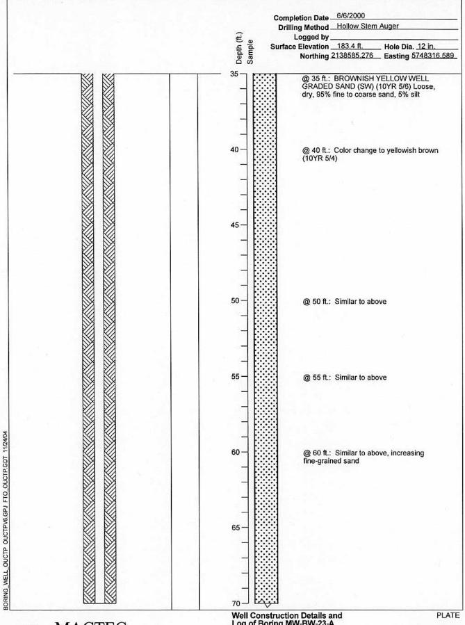
Well Construction Details and Log of Boring MW-BW-23-A
