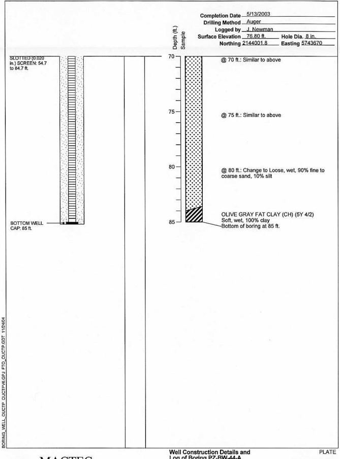
Well Construction Details and Log of Boring PZ-BW-44-A
