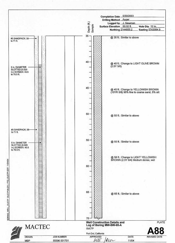
5/30/2003 Completion Date -Drilling Method Auger Depth (ft.) Sample Logged by \_\_J. Newman Surface Elevation 50.02 ft. Hole Dia. 12 in. Northing 2144855.2 Easting 5743084.9 OLIVE FAT CLAY (CH) (5Y 5/4) Firm, moist, 95% fat clay, 5% fine sand -Bottom of boring at 71 ft. End cap to bottomof screen: 5 in. BOTTOM WELL CAP: 71 ft. Hole cleaned out to 71 ft. BORING\_WELL\_OUCTP OUCTPV6.GPJ FTO\_OUCTP.GDT 11/24/04 Well Construction Details and Log of Boring MW-BW-65-A PLATE MACTEC
